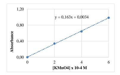
Figure 1. Calibration curve of KMnO<sub>4</sub>
